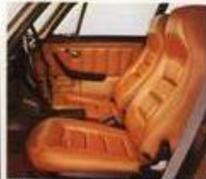
The bucket seats adjust forward, backward, up-down. The backrests swing from upright to horizontal. Lumber support is adjustable. Seats are covered in leather.
