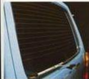
Visibility is unusually good through the back window because it's equipped with an electrically-heated defroster and its own wiper and washer.
